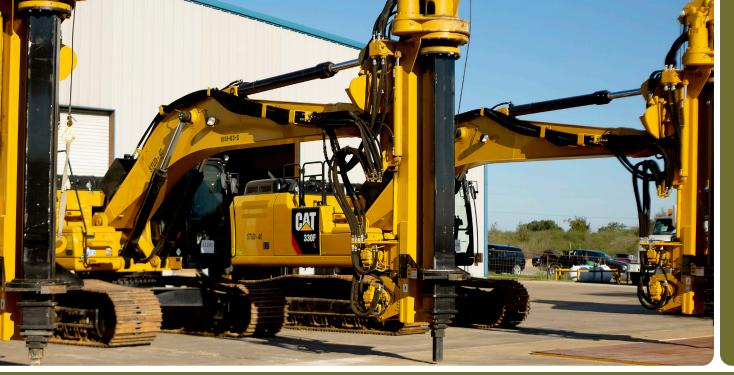
The **Spiradrill Topdrive Utility Drill (STUD)** is an excavator-mounted drill designed to deliver increased drilling power and maneuverability in difficult working conditions. The low operational height is ideal for low clearance jobs such as under existing power lines or structures.
