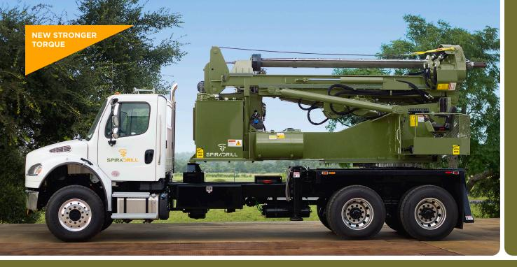
The **LHD series** is the premier drill in its class. The unique crowd design allows the mast, winch, Kelly, and rotary gearbox to feed the drill tool simultaneously, making it easier, safer, and more efficient. The LHD is available in several different models, including a "Short Mast" road-legal truckmounted unit, and a track-mounted unit. This versatile unit has the increased capacity and ability to drill larger diameter holes in even the toughest soil conditions.
